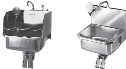
Same construction and features of the pedestal sink, but equipped with instant action stainless steel knee pedal valve. Ideal where floor maintenance is a prime concern. Also available with side walls for protection against contamination of food items when hand lav is close to processing tables. Overall dimensions 20" x 18" x 16".
